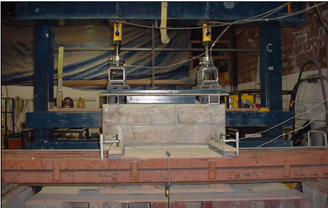
Figure 2: Photograph of the Redi-Rock blocks in the shear test frame
