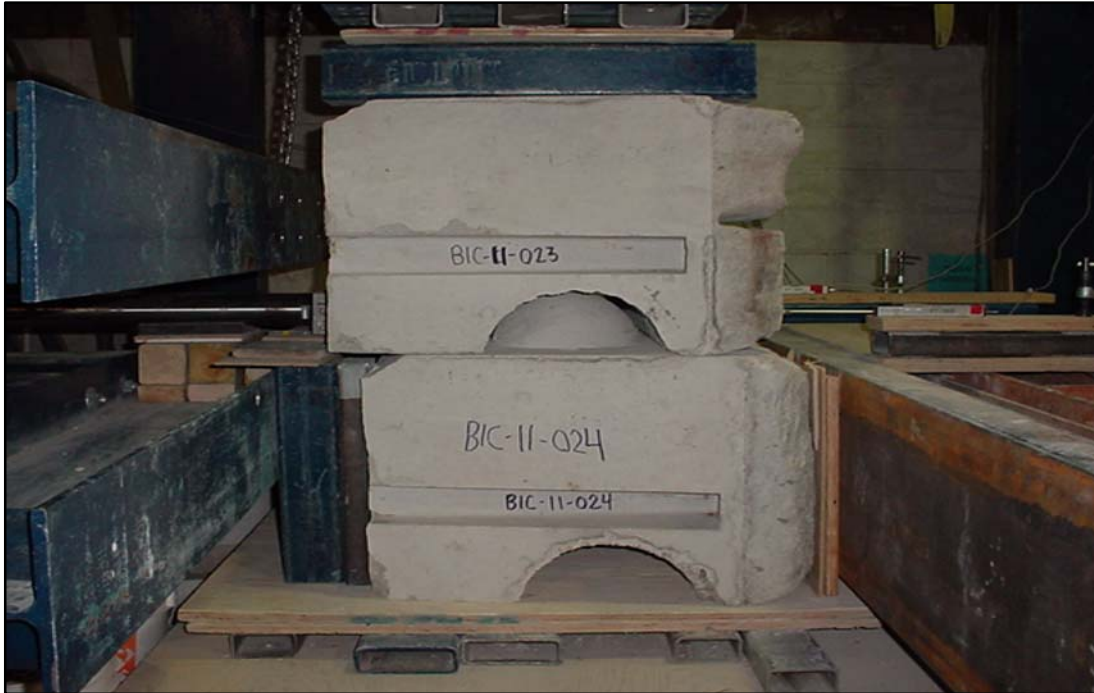
Figure 1: Photograph of the Redi-Rock blocks in the shear test frame
