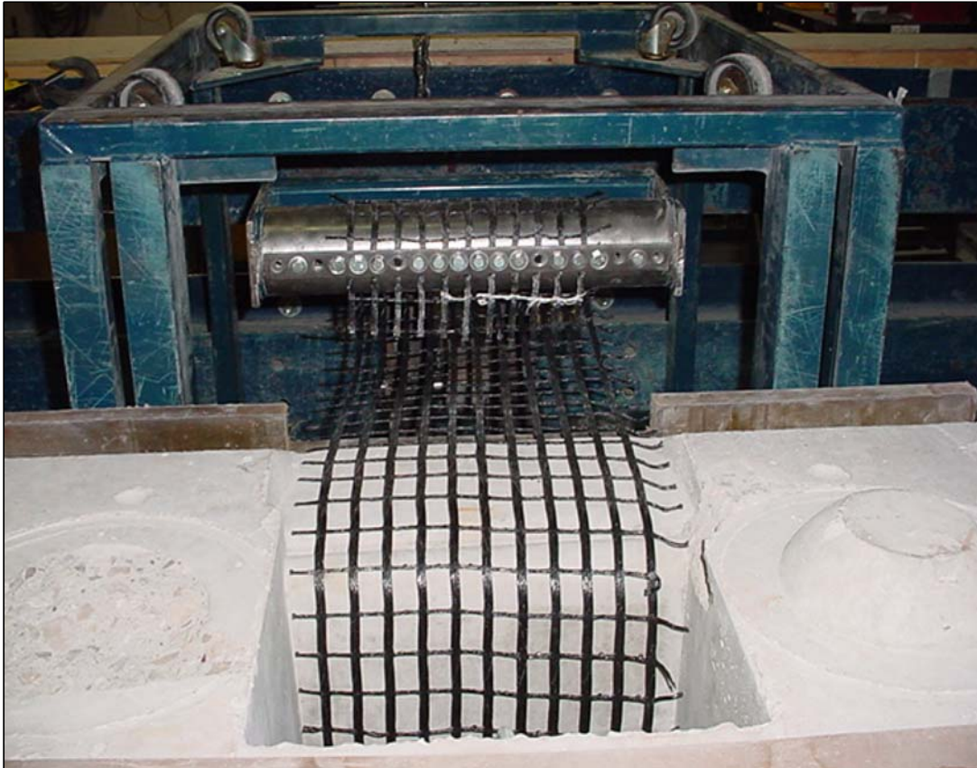
Figure 3: Photograph of the Redi-Rock Positive Connection (PC) Block system and Miragrid 10XT geogrid
