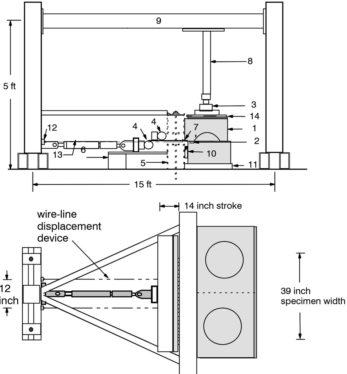
Figure 1: Schematic of connection test apparatus showing Redi-Rock units and Miragrid 5XT geogrid using the anchored tail configuration
