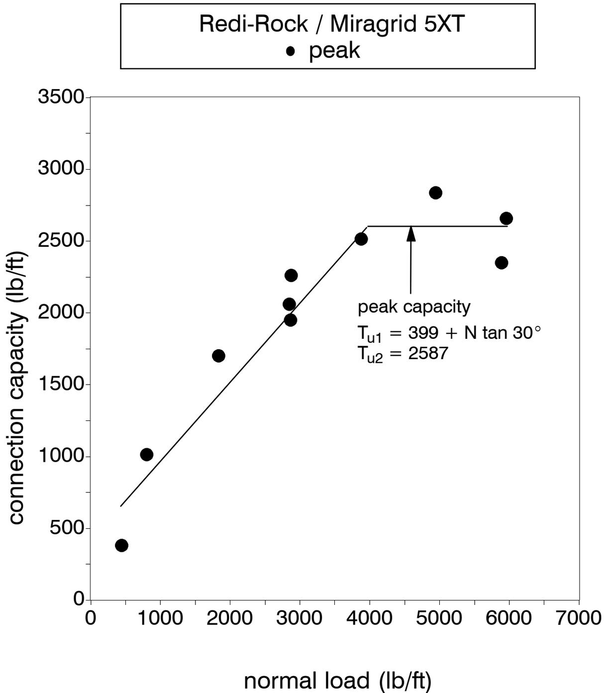
Figure 3: Connection capacity versus normal load for Redi-Rock block with one 7/16 inch diameter fiberglass connector rod and Miragrid 5XT using the anchored tail configuration
