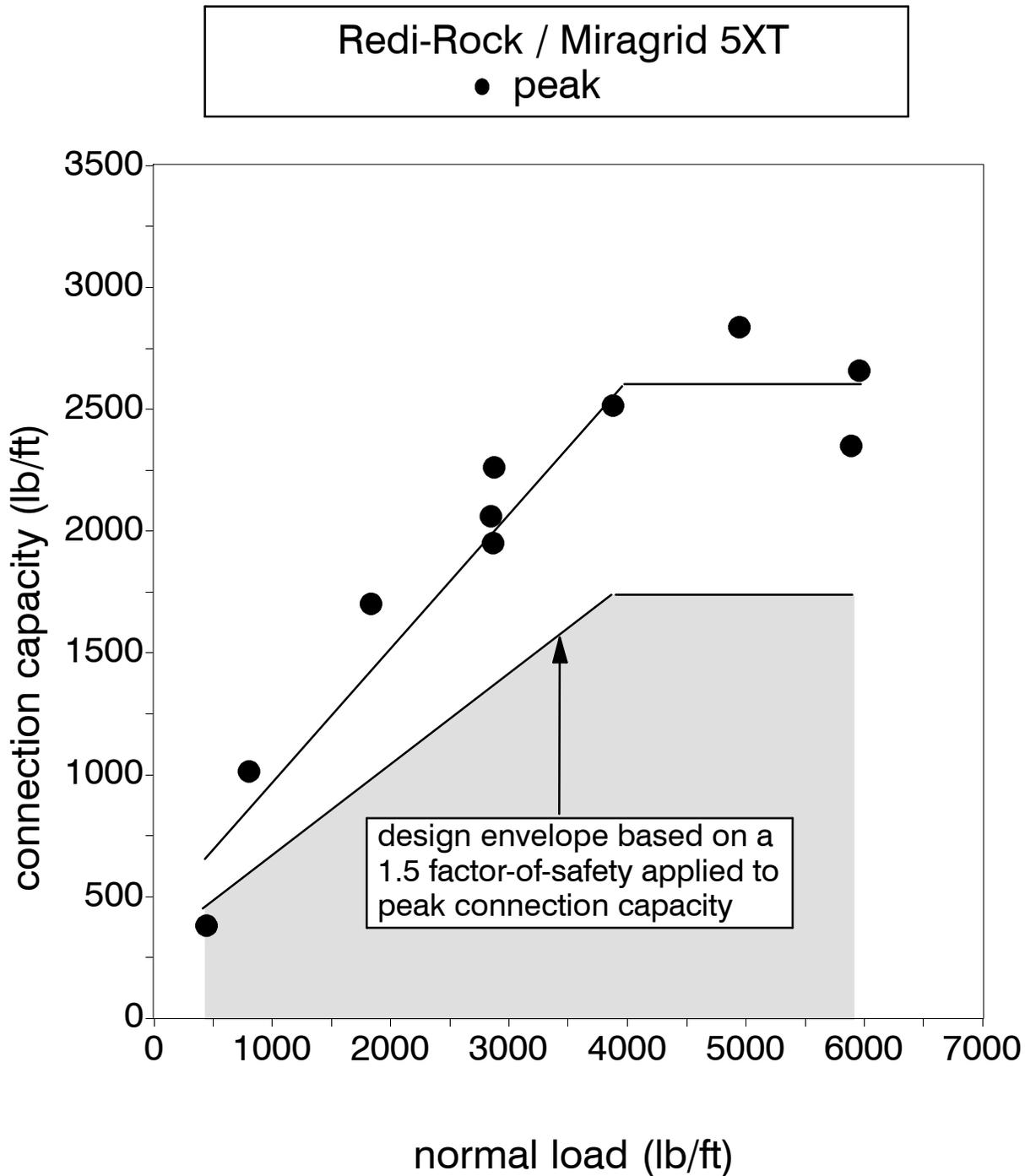
Figure 4: Preliminary design capacity envelope for Redi-Rock modular block units with one 7/16 inch diameter connector rod and Miragrid 5XT geogrid combination using the anchored tail configuration
