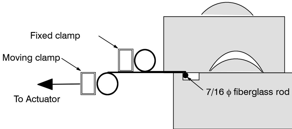
Figure 2: Schematic of connection detail and clamp arrangement
